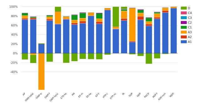
As shown in the figure below, the raw material supply (A1) dominates in most environmental core indicators. The highest influence on the Global Warming Potential (GWP-total) have raw material supply (A1). Transports (A2, C2) and waste processing (C3) have rather a minor impact within all core indicators.
